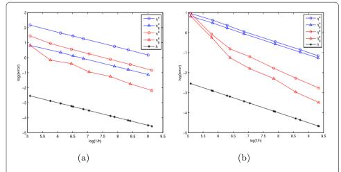
**Figure 3** The convergence rate of adaptive and uniform refinements for the problem on L-shape domain with slip boundary condition: g is continuous at (0,0). (a):  $P_1 - P_0$ ; (b):  $P_1 - P_1$
