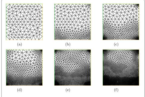
**Figure 10** Adaptive refinements by  $\mathbf{P}_1 - P_1$  stabilized method for the cavity flow with slip boundary condition: g = 100.0. (a):  $\mathcal{T}_1$ ; (b):  $\mathcal{T}_2$ ; (c):  $\mathcal{T}_3$ ; (d):  $\mathcal{T}_4$ ; (e):  $\mathcal{T}_5$ ; (f):  $\mathcal{T}_6$
