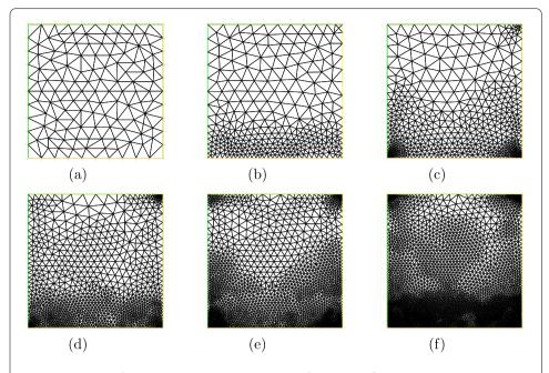
**Figure 7** Adaptive refinements by  $\mathbf{P}_1 - P_0$  stabilized method for the cavity flow with slip boundary condition: g = 100.0. (a):  $\mathcal{T}_1$ ; (b):  $\mathcal{T}_2$ ; (c):  $\mathcal{T}_3$ ; (d):  $\mathcal{T}_4$ ; (e):  $\mathcal{T}_5$ ; (f):  $\mathcal{T}_6$
