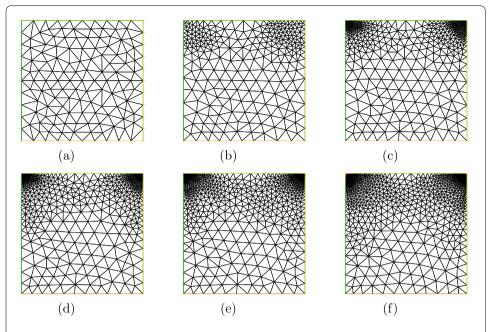
**Figure 5** Adaptive refinements by  $\mathbf{P}_1 - P_0$  stabilized method for the cavity flow with slip boundary condition: g = 1.0. (a):  $\mathcal{T}_1$ ; (b):  $\mathcal{T}_2$ ; (c):  $\mathcal{T}_3$ ; (d):  $\mathcal{T}_4$ ; (e):  $\mathcal{T}_5$ ; (f):  $\mathcal{T}_6$
