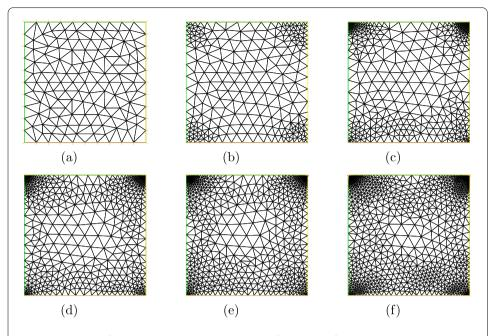
**Figure 9** Adaptive refinements by  $\mathbf{P}_1 - P_1$  stabilized method for the cavity flow with slip boundary condition: g = 10.0. (a):  $\mathcal{T}_1$ ; (b):  $\mathcal{T}_2$ ; (c):  $\mathcal{T}_3$ ; (d):  $\mathcal{T}_4$ ; (e):  $\mathcal{T}_5$ ; (f):  $\mathcal{T}_6$
