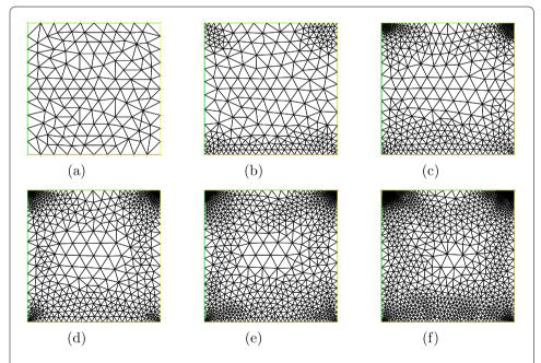
**Figure 6** Adaptive refinements by  $\mathbf{P}_1 - P_0$  stabilized method for the cavity flow with slip boundary condition: g = 10.0. (a):  $\mathcal{T}_1$ ; (b):  $\mathcal{T}_2$ ; (c):  $\mathcal{T}_5$ ; (d):  $\mathcal{T}_6$ ; (f):  $\mathcal{T}_6$
