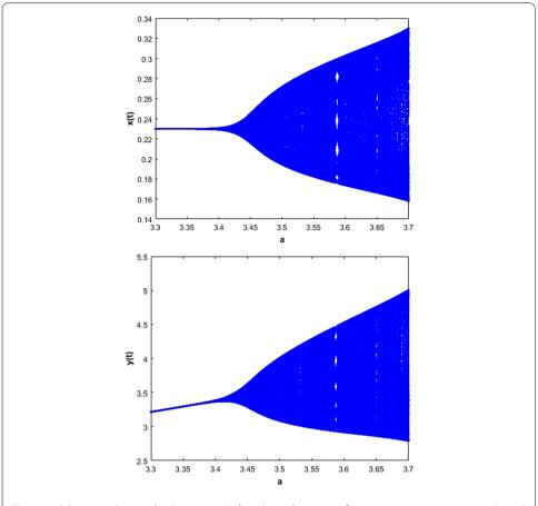
**Figure 2** Bifurcation diagram for the system (2) for values of m = 0.25,  $\beta = 0.23$ , a = 3.3:0.0001:3.4 and initial value  $(x_0, y_0) = (0.2, 3.4)$
