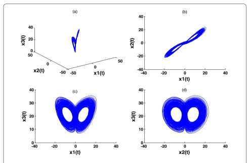
**Figure 1** Chaotic attractors of the fractional-order unified system: (**a**) plot in the  $(x_1, x_2, x_3)$ -space; (**b**) plot in the  $(x_1, x_2)$ -plane; (**c**) plot in the  $(x_1, x_3)$ -plane; (**d**) plot in the  $(x_1, x_2)$ -plane
