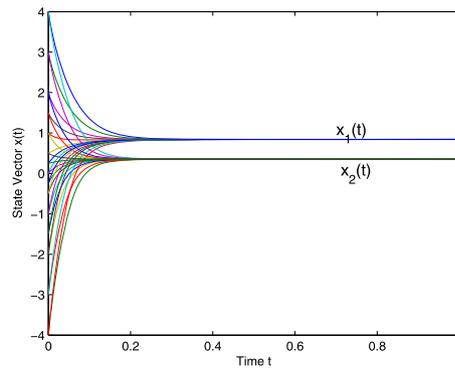
**Figure 3** The state trajectory  $x$  of neural network (17) in Case 3 of Example 1.
