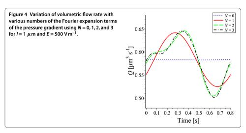
in the microchannel of elliptic cross-section when the flow is evidently driven by both the pulsatile pressure gradient and the electrokinetic force.
