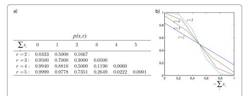
Figure 3 (a) Table representing the values of p(r, x) for several values of  $r \in \mathbb{N}$  and  $x \in \{0, 1\}^k$ . (b) For different values of r, x, the probability that g(x) = 0 if a cooperative function g of r inputs is randomly sampled.
