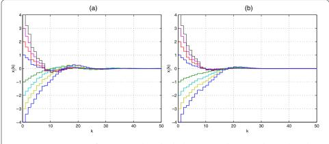
Figure 2 State trajectories of Case 1: (a) With randomly changing coupling strength,  $\rho_m c$ ; (b) With fixed coupling strength, c (Example 1).
